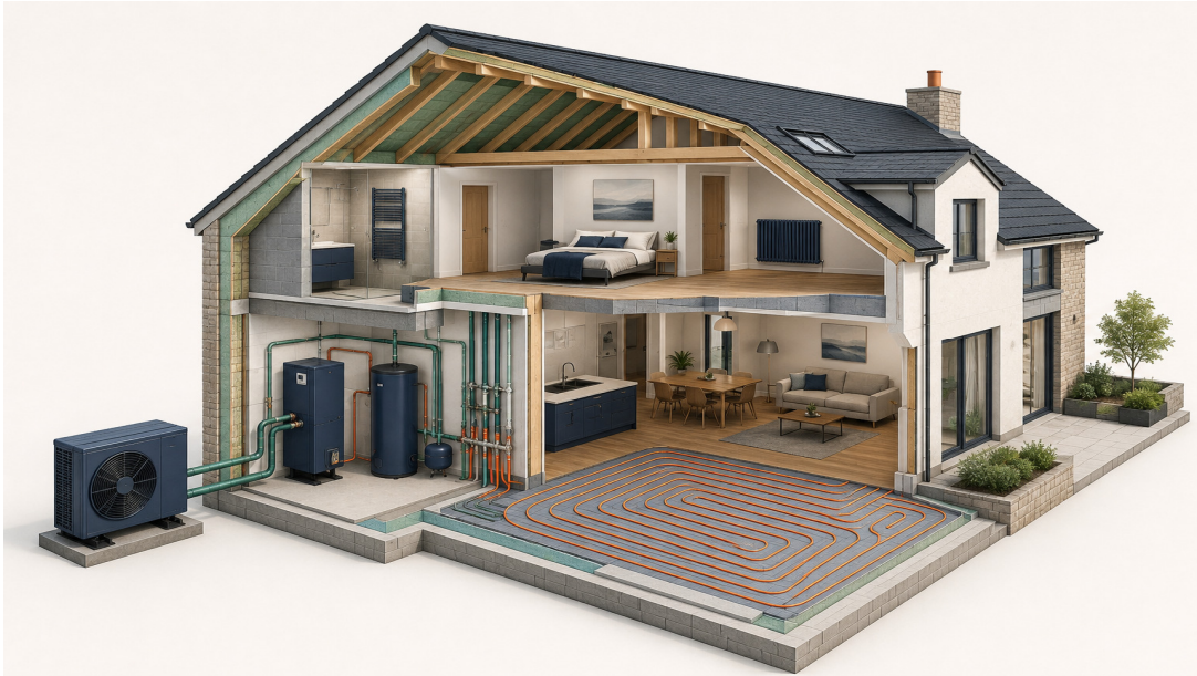
Figure 1 – Principal components of an air-to-water heat pump serving a domestic heating system.
