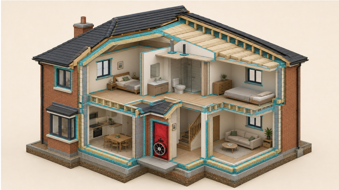
Figure 1 – Complete dwelling with continuous air barrier and blower-door test setup.
