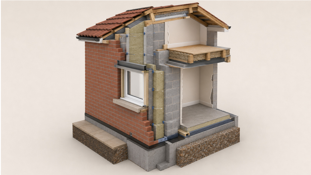
Figure 1 – Typical modern insulated masonry cavity-wall construction.
