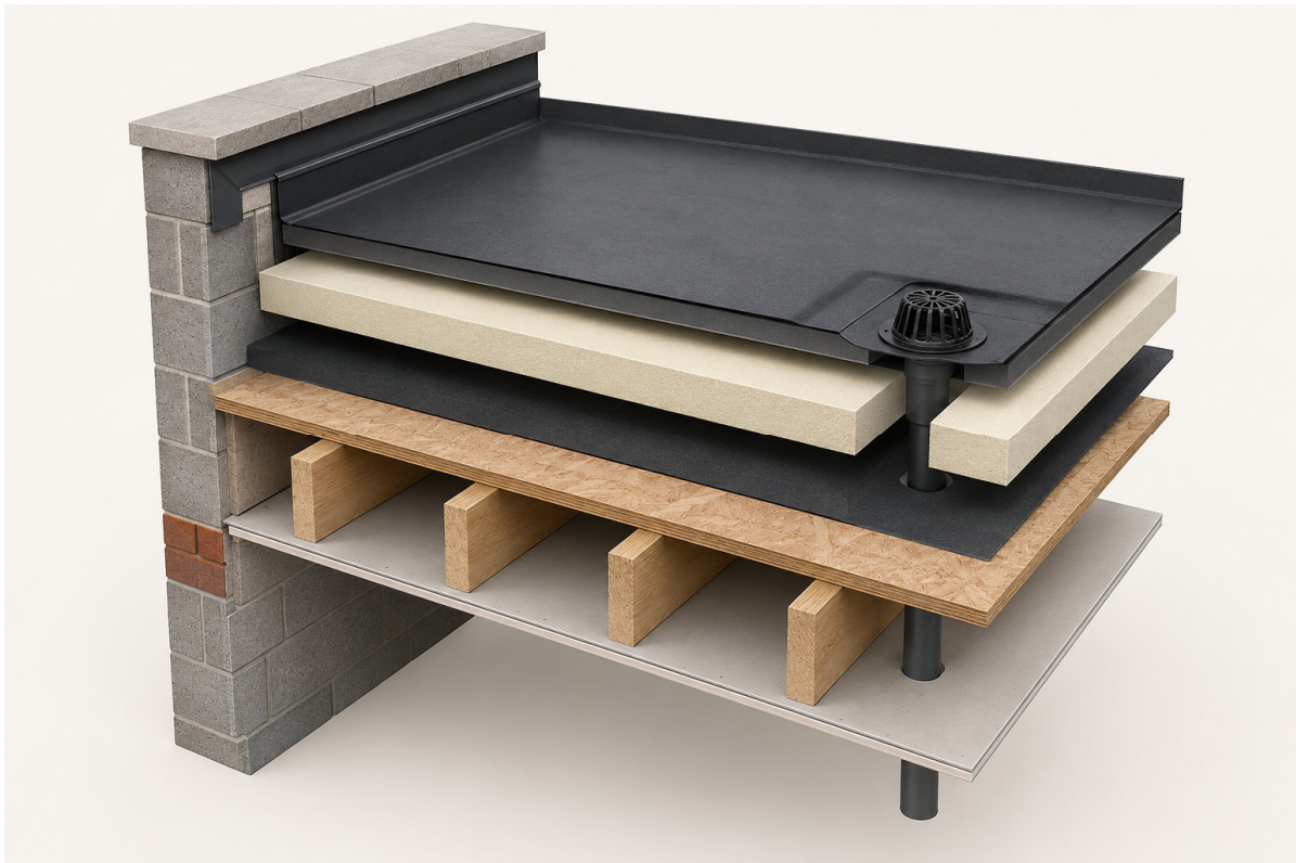
Figure 1 — Warm flat roof with its weatherproofing, insulation, outlet and supporting structure exposed.
