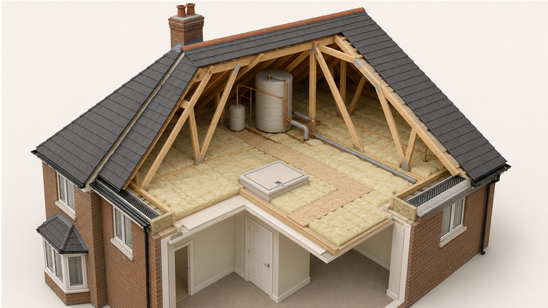
Figure 1 – Typical insulated domestic loft with services and ventilation zones exposed.
