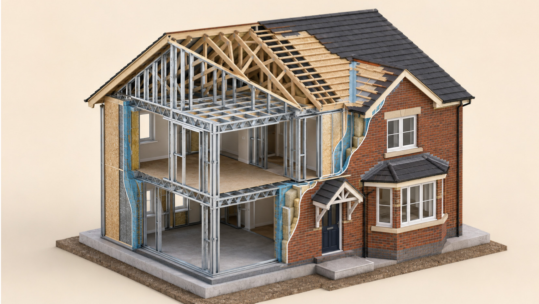
Figure 1 – Typical two-storey light-gauge steel-framed domestic construction.
