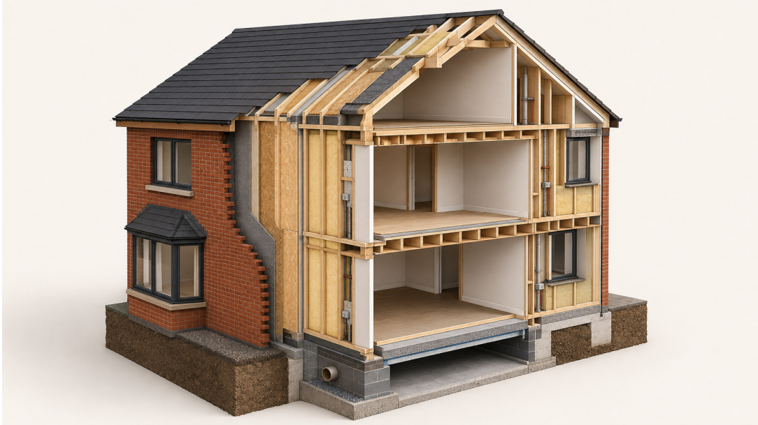
Figure 1 – Typical two-storey platform timber-frame house construction.
