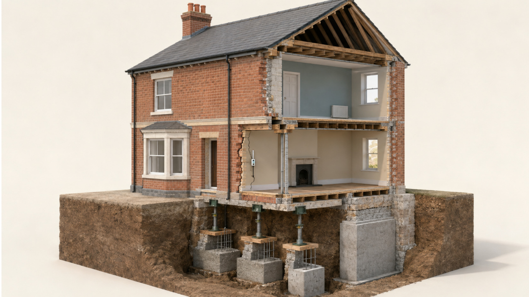
Figure 1 – Traditional staged underpinning transfers an existing wall to deeper competent ground.
